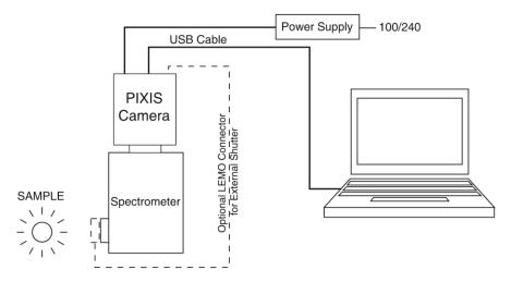
Figure 3. Typical Spectroscopy Experiment Layout (Air-cooled Camera)
